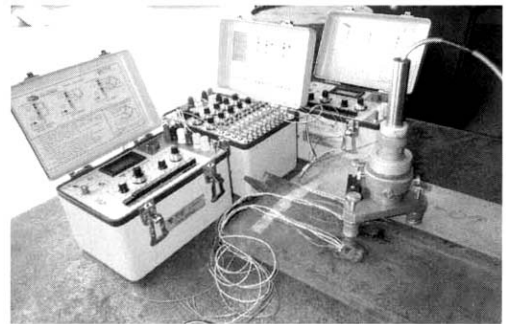
Fig. 4. Configuration of instrument on residual strain measurement.
