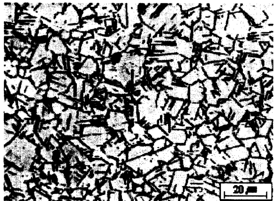
Fig. 3. Alloy718 showing the distribution of \delta phase at grain boundaries.
