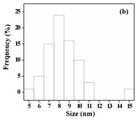
**Figure 2.** (a) TEM pictures of platinum nanoparticles synthesized using a 1:40 concentration ratio of  $K_2PtCl_4$  to acrylic acid at room temperature and (b) size distribution of cubic nanoparticles.
