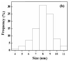
Figure 1. (a) TEM images of platinum nanoparticles prepared using a 1:5 concentration ratio of K<sub>2</sub>PtCl<sub>4</sub> to polyacrylate at room temperature and (b) their size distribution.
