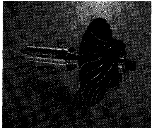
Fig. 1 Centrifugal impeller and motor rotor assembly
