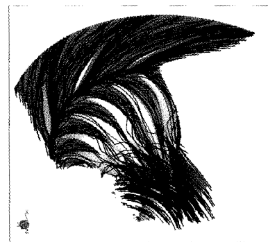
Fig. 6 Streamlines in three-dimensional passage ( \dot{m} = 0.286 \text{ kg/sec} )
