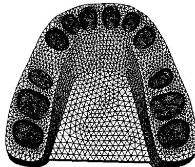
Fig. 7 Finite element model of alveolar bone
