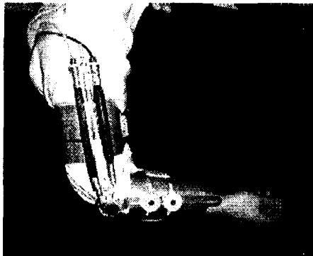
Fig 3. Assistive device to support elbow motion using air muscle actuators
