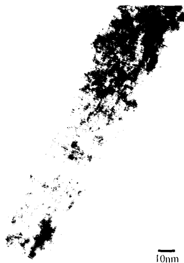
Fig. 6. TEM image for one of the carbon nanofibers under 80 Torr total pressure condition.
