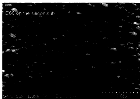
Fig. 3. FE-SEM top view of pure fullerite film on silicon substrate.
