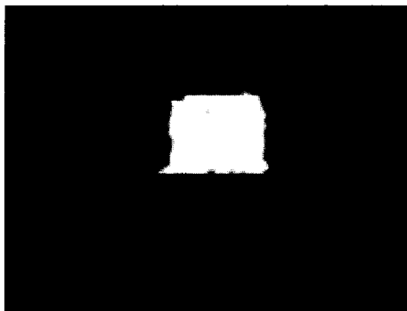
Figure 5. The near field pattern of a covered ridge waveguide.
