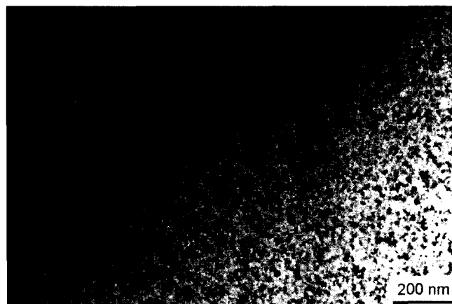
Fig. 6. Structure of (Fe_{0.5}Co_{0.5})_{86}Hf_7Cu_1B_6 alloy after nanocrystallisation at 575 °C and long-term annealing at 500 °C. Bright field image.
