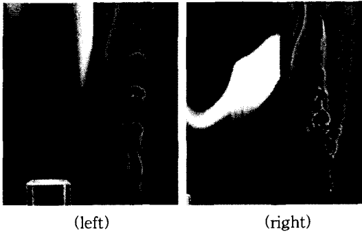
Fig. 9(a) Representative direct photo and schlieren image in regime 2 ; 40% C 3 H 8 / 60% N 2 , U 0 =1.5m/s, (left) U f /U 0 =0.88 (right) U f /U 0 =1.88
