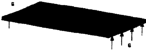
Fig. 3 Shock test condition (220G, 2msec)
