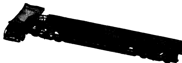
Figure 8. Deformed shape at head-on collision.
