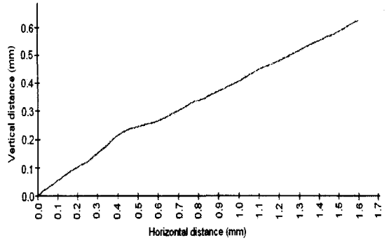
(b) Measured surface profile of the casting part at 15 deg.
