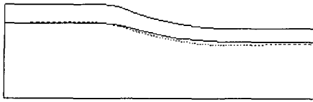
Fig. 12 Cu-Al contact profile in an Eulerian mesh before and after correction using a stream line technique
