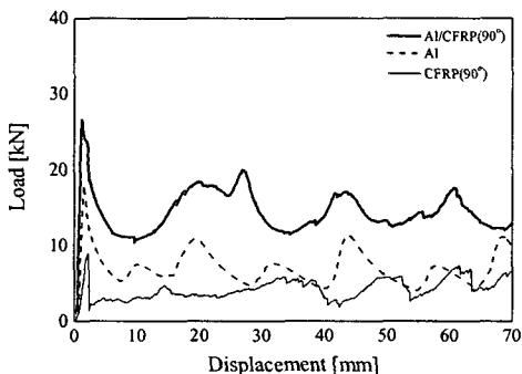
Fig. 5 Load-displacement curve of square tubes
