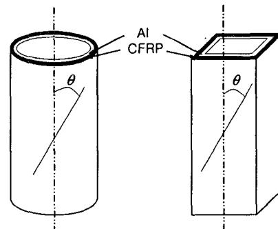
Fig. 1 Configuration of Al/CFRP compound tube
