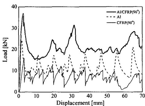
Fig. 4 Load-displacement curve of circular tubes
