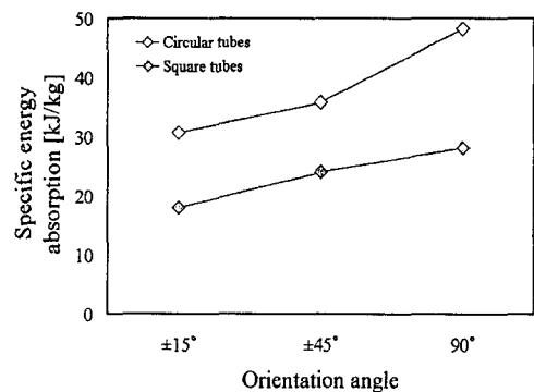
Fig. 7 Specific energy absorption of Al/CFRP compound tubes with the different orientation angle
