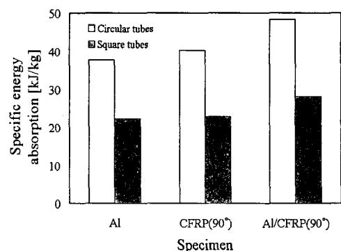
Fig. 6 Specific energy absorption of square and circular tubes
