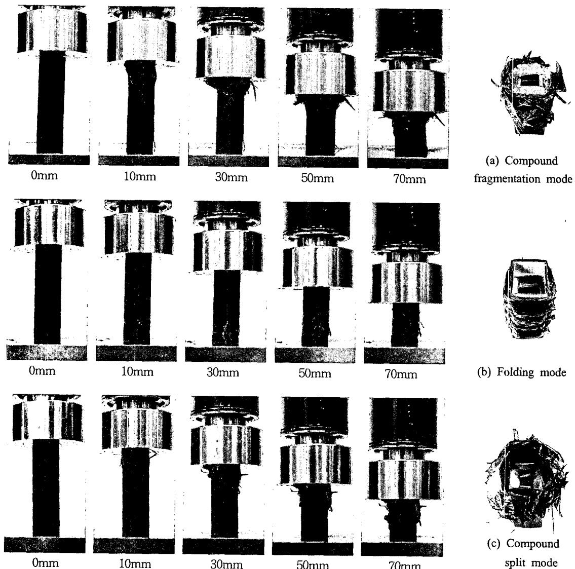
Fig. 3 Collapsing process and typical collapse modes of Al/CFRP compound square tubes
