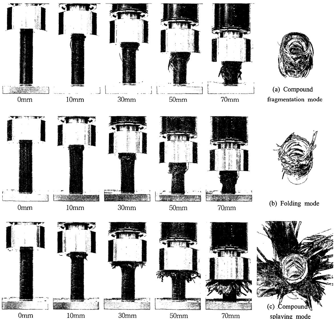
Fig. 2 Collapsing process and typical collapse modes of Al/CFRP compound circular tubes
