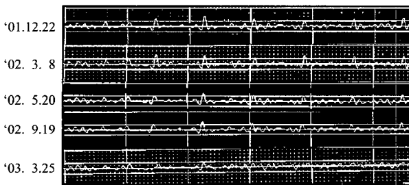
Fig. 5. The Vertical Track Settlement Progress on Bridge
