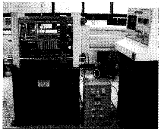
Fig. 2 The photo of hot metal extru-bending machine
