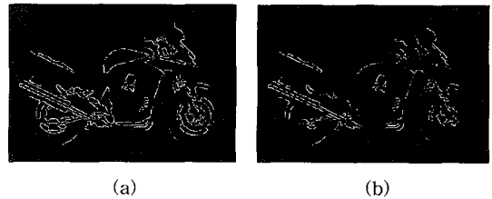
Fig. 2. Energy of the edge direction histogram can be increased by eliminating circular edge pixels. Left and right images show edge pixels before and after elimination of the edge pixels, respectively. The energy of left and right image is 0.026 and 0.037, respectively.
