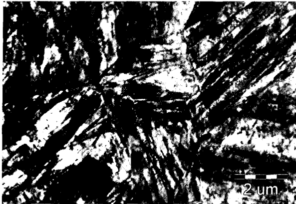
Fig. 1. Transmission electron micrograph showing bainitic lath of the 6.5Mn hot rolled steel sheet.
