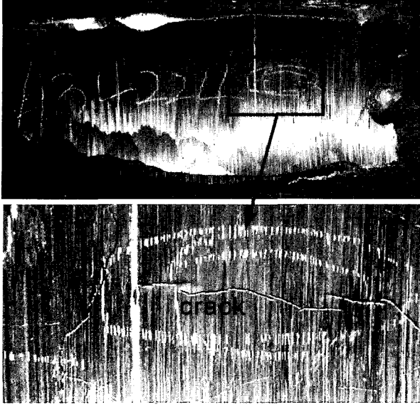
Fig. 1. Cracks on ingot surface.
