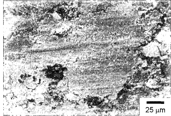
Fig. 6. Scanning electron microphotographs of the surface in specimen prepared in the experimental procedure of N90 followed by the frictional test.
