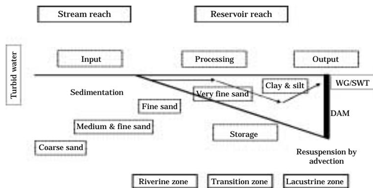
**Fig. 5.** Dynamics of turbid water after the monsoon rainfall in Hoingsong Reservoir applicable selective withdrawal discharge. WG: watergates, SWT: selective withdrawal tower.
