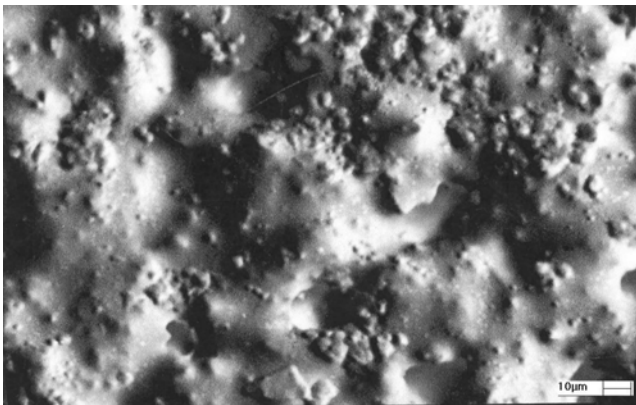
Fig. 2. SEM photograph of C-SiC-B 4 C composites of D-1 batch, upon oxidation in air at 800 °C for 1h.
