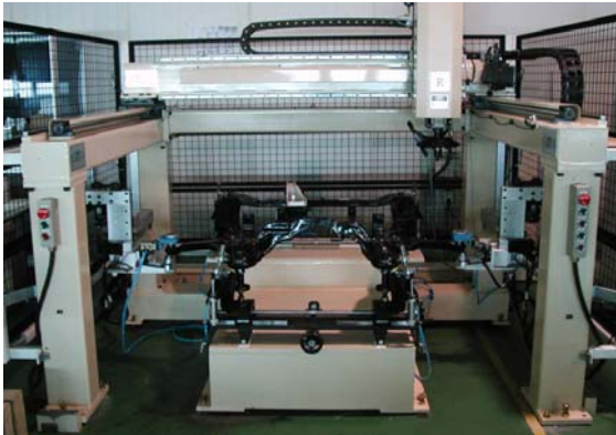
Fig. 5 Inspection system for sub-frame
