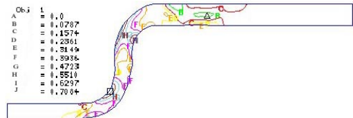
(b) Effective strain of 2nd-drawing
