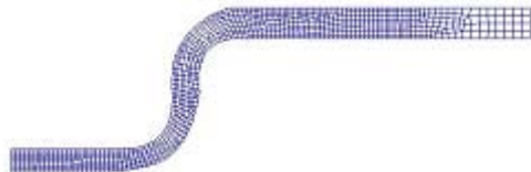
(b) Mesh deformation of 2nd-drawing
