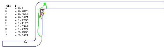
(e) Effective strain of 5th-drawing
