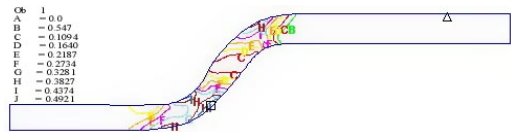
(a) Effective strain of 1st-drawing
