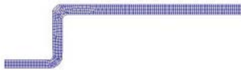
(e) Mesh deformation of 5th-drawing
