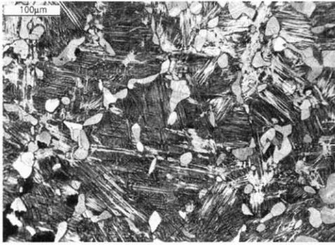
Fig. 2b. Optical micrograph showing the microstructure of the bronze vessel shown in Fig 2a.
