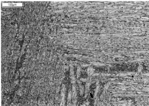
Fig. 5a. Optical micrograph showing the as - cast microstructure of the Cu - 24wt%Sn alloy.
