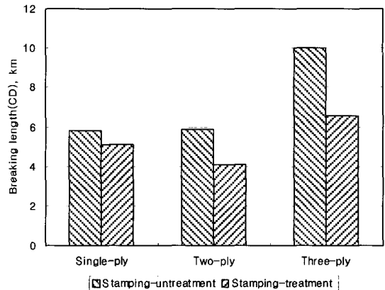
Fig. 11. Changes of breaking length of Hanji sheets by stamping treatment.
