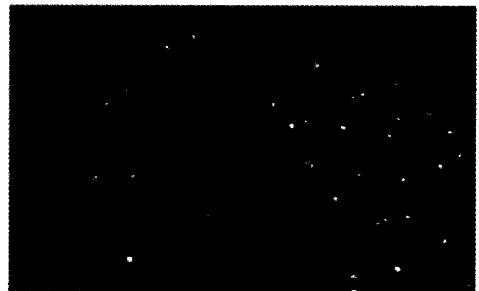
(b) Near Wall TIRFM Image with \theta_i = 65^\circ ( z_p = 114 nm)
