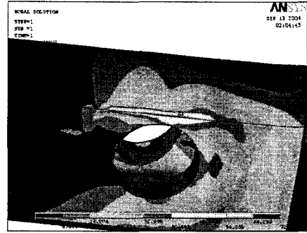
Fig. 6 FEM analysis result of rocker arm shaft
