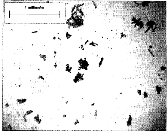
Fig. 4. Image of MMS after agitating at distilled water of 45°C.
