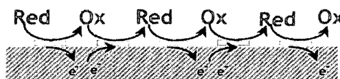
Fig. 1. Concept of conventional planar IDA electrode and redox recycling of electroactive species
