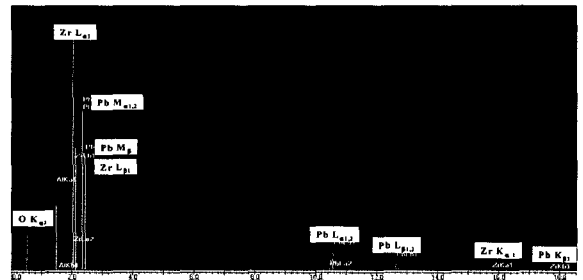
[그림 3] a) Top view of PbZrO 3 bundles and thin film which illustrated the formation of open tubes with an outer diameter of 200nm and thin film in the portion of surfaces. b) Energy dispersive X-ray spectrometric analysis with the presence of (Pb, Zr) on PbZrO 3 bundle.
