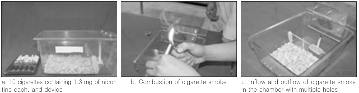
Fig. 1. Specifically designed cigarette smoke device, 45×20×20 cm 3 sized clear acrylic resin chamber
