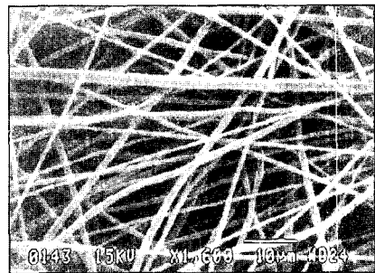
PGA scaffold fabricated by electrospinning
