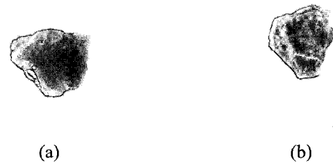
Fig. 1. A photograph of African rubies (a) non-treated and (b) heat-treated at 1500°C for 12 hrs in O 2 gas.
