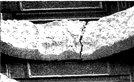
Fig. 3. SEM of beam lead crack in TCP.
