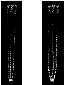
Fig. 7 Lead deformation with respect to lead geometry of linear lead (left) and bent lead (right)
