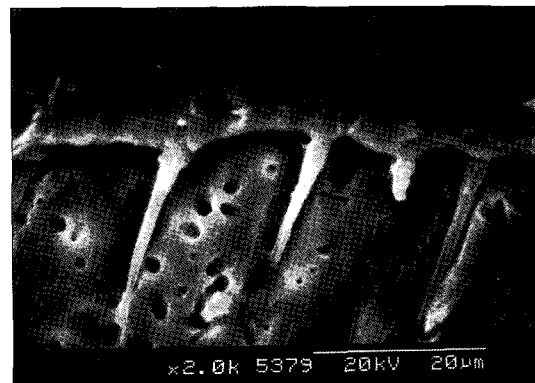
Figure 8. SEM photograph of the adhesive interface of BI-AB. Hybrid layer is well formed and resin tags are infiltrated into dentinal tubules deeply.
