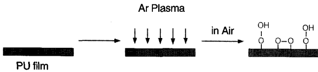
Figure 2. Schematic representation of Ar plasma treatment.
