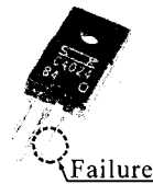
(b) Failure of chip lead frame by thermal stress Fig. 2 Failure of BLDC motor by temperature and thermal stress.
