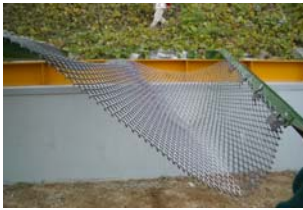
(a) Rockfall energy 50KJ(Weight : 0.4ton, Height : 12.5m)
