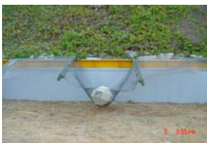
(c) Rockfall energy 50KJ(Weight : 0.25ton, Height : 22m)
