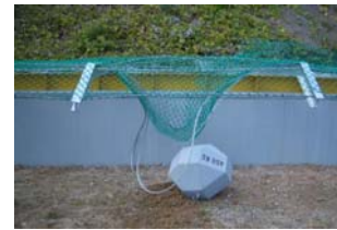
(b) Rockfall protection fence damage(rockfall energy=50 kJ)
