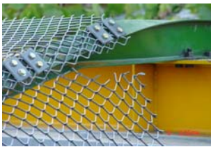
(b) Damage at bolting section
