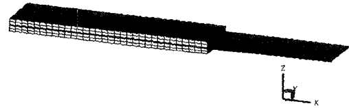
Fig. 5 Meshed piezoelectric cantilever shape generated from auto-mesh generator ( 26 \times 4 \times 1.1 mm)
