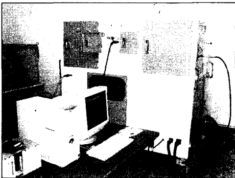
Fig. 5 Configuration of Water Pressure Test Facility
