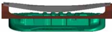
Fig. 4 Gravity sink material inflow
