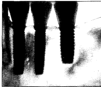
Fig. 28. Stresses produced by loading on distal fossa of posterior implant in G3.
