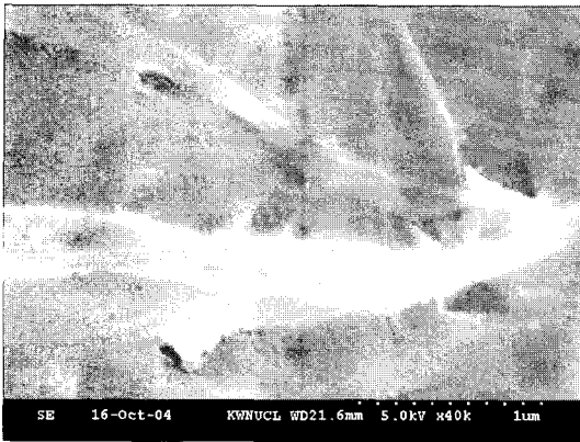
Fig. 10. High resolution SEM image of sheet surface sprayed with 1% CNS. (magnification x50,000)
