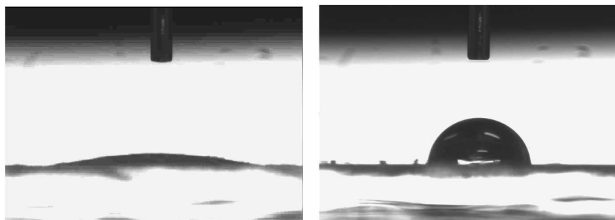
Figure 3. Water contact angles of microcrystalline layer on vinyl tape (left) and simple vinyl tape (right).
