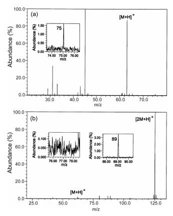
**Figure 4**. Electron ionization mass spectra of ethylene glycol at 70 eV of the electron ionization energy. The sample pressures and ion trapping times are  $3.0 \times 10^{-6}$  Torr and 50 ms (a)  $4.0 \times 10^{-6}$  Torr and 10 s (b).
