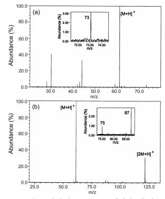
**Figure 2**. Electron ionization mass spectra of ethylenediamine at 70 eV of the electron ionization energy. The sample pressures and ion trapping times are  $3.0 \times 10^{-6}$  Torr and 50 ms (a)  $4.0 \times 10^{-6}$  Torr and 10 s (b).
