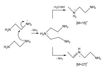
Scheme 2. Formation of  $[M+15]^+$  and  $[M+27]^+$  by ion-molecule reaction.
