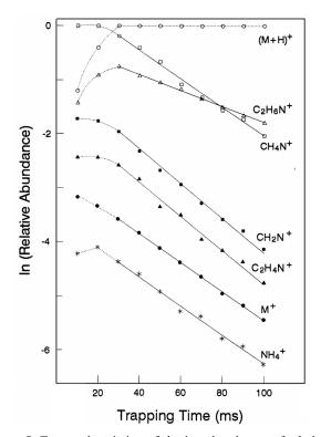
**Figure 5**. Temporal variation of the ion abundances of ethylenediamine. The electron ionization energy of 70 eV and the sample pressure is about  $3.0 \times 10^{-6}$  Torr.
