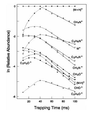
Figure 6. Temporal variation of the ion abundances of ethanolamine. The electron ionization energy of 70 eV and the sample pressure is about  $3.0 \times 10^{-6}$  Torr.
