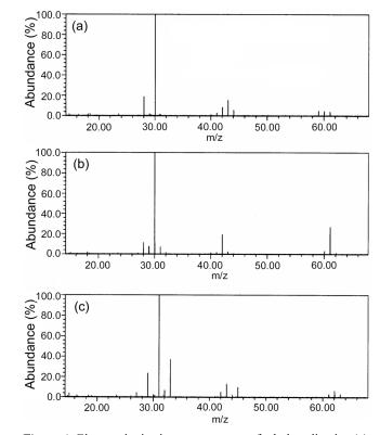
**Figure 1**. Electron ionization mass spectra of ethylenediamine (a), ethanolamine (b), and ethylene glycol (c) at the electron ionization energy of 70 eV and the ion trapping time of 1 ms. The pressures are about  $3.0 \times 10^{-6}$  Torr.
