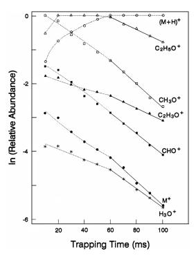
**Figure 7**. Temporal variation of the ion abundances of ethylene glycol. The electron ionization energy of 70 eV and the sample pressure is about  $3.0 \times 10^{-6}$  Torr.
