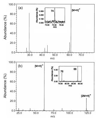
**Figure 3**. Electron ionization mass spectra of ethanolamine at 70 eV of the electron ionization energy. The sample pressures and ion trapping times are  $3.0 \times 10^{-6}$  Torr and 50 ms (a)  $4.0 \times 10^{-6}$  Torr and 10 s (b).
