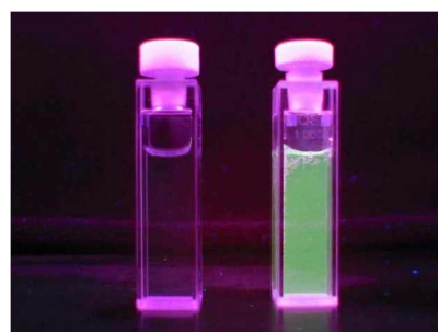
Figure 1. Photograph of polysilole in THF (10 mg/L, left) and polysilole nanoaggregates in water-THF mixture (90 : 10 by volume, 10 mg/L, right) under blacklight.
